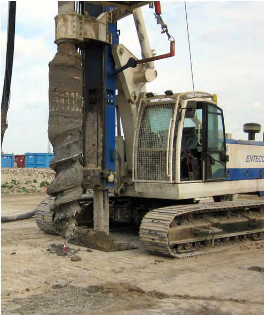
ENTEKO E6050 MODEL EQUIPPED WITH SOIL DISPLACEMENT APPLICATION
