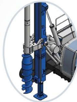
SP Soil Displacement
